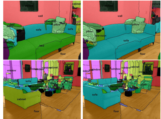
Fig. 4: Examples illustrating where object detectors and scene classification help: Semantic segmentation output improves as we add features from object detector activations and scene classifiers (going from left image to right image).
